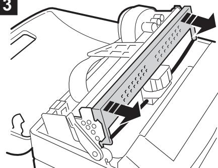
**GB** **Replacing the ribbon cartridge**
