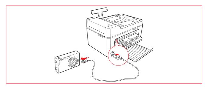
The green USB status LED illuminates to indicate that a correct connection has been established. If the connection is not established, make sure you have connected a compatible device.
