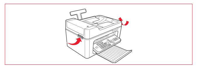
Press the lever to remove the ink cartridge you want to replace.
