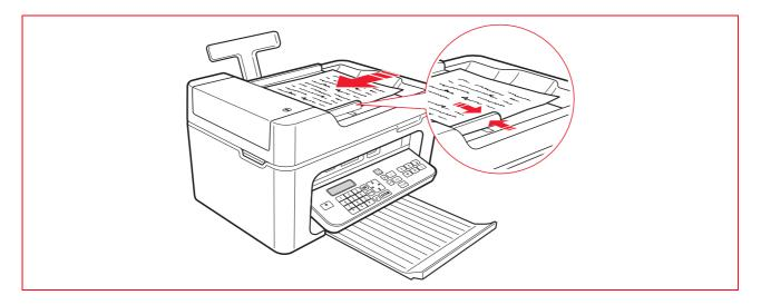
2 Adjust the paper width guide of the automatic document feeder and make sure that it is positioned against the edge of the paper.
