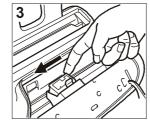
Move the print cartridge carriage to the left-hand edge of the fax machine.
