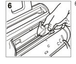
6. Clean the glass surface of the optical reader with a cloth dampened with a product designed specifically for cleaning glass and then dry it thoroughly. Warning!
