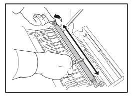
5 Put away the cleaning brush, press the specified position of the front cover and left cover 1 to close.
