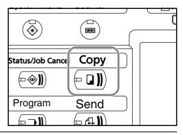
**NOTE:** If you place the original and press the **Start** key before the copier has warmed up, only the scanning is performed in advance and the copying job starts upon completion of the warm-up.
