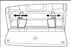
3 Insert the paper along the paper width guides into the tray until it stops.
