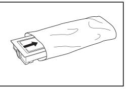
21 Unwrap a new toner container and hold the new toner container upright and tap the top of the container 5 or more times.
