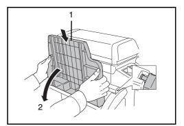
7 Turn the lever to lower the finisher process tray.
