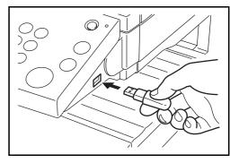
**IMPORTANT:** Use USB memory formatted by this machine. If a USB memory formatted by any other device is used, *Removable Memory is not formatted*. may appear. To format a USB memory, press [Format] and follow the instructions on the screen.
