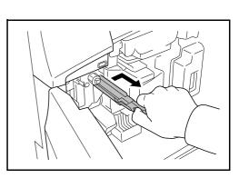
8 Take the grid cleaner provided out of its bag and remove the cap.
