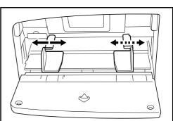
**3** For landscape form envelopes, close the flap. Insert the envelope all the way along the width guides, keeping the printing side face-up and with the flap closed.
