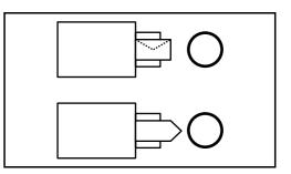
**IMPORTANT:** How to load envelopes (orientation and facing) will differ depending on the type of envelope. Be sure to load it in correctly, otherwise printing may be done in the wrong direction or on the wrong face.
