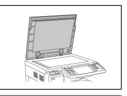
**NOTE:** If the optional document processor is installed, open the document processor. Before opening the document processor, be sure that there are no originals left on the original table or on the original eject table. Originals left on the original table or on the original eject table may fall off when the document processor is opened.
