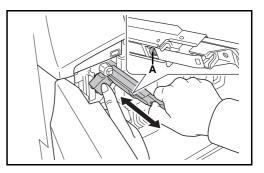
**CAUTION:** When pushing the main charger back in, take care not to push it all the way in. This could result in damage to copies.
