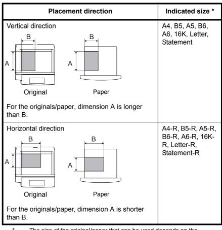
The size of the original/paper that can be used depends on the function and source tray. For further details, refer to the page detailing that function or source tray.
