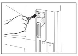
**3** Connect the other end of the cable to the PC.
