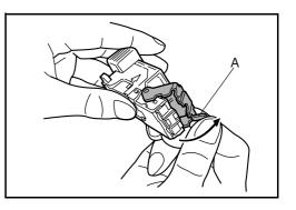
3 Clear the staple jammed in the cartridge end (staple-loaded side).
