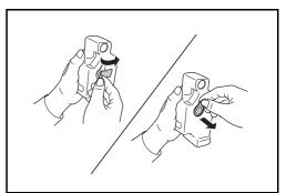
4 Fit the cap into the opening in the waste toner box and attach the sticker over the cap.
