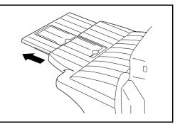
• The paper sizes are marked on the finisher tray extension. Open ejected paper guides 1 and 2 as necessary to match the paper size.
