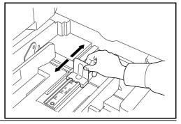
**NOTE:** Paper sizes are indicated on the cassettes. To change between inch size and metric size (A, B sizes), follow the steps below to adjust the size switch.
