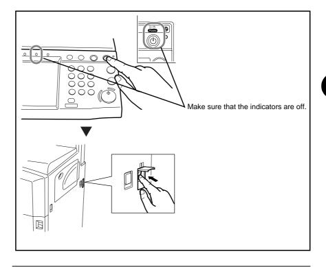
**IMPORTANT:** Do not turn the main power switch off when the optional fax kit is installed. If you turn the main power switch off, you cannot receive fax messages.
