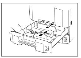
**3** Using the paper length guide, move the plate to fit the paper.
