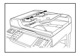
2 Place the originals. Put the side to be scanned (or the first side of two-sided originals) face-up. Slide the leading edge into the document processor as far as it will go. The original placement indicator will be lit.
