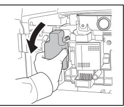
**3** Peel the sticker off the waste toner box and remove the cap.
