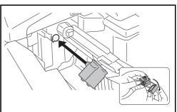
10 While gently holding the grid cleaner in place with your left hand, pull the main charger out fully and then push it back to a position where the roller A does not quite reach the white pad on the grid cleaner. Repeat this procedure 2 or 3 times.
