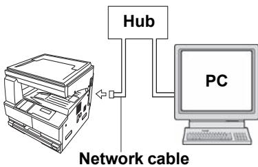
Connecting the scanner to your computer network with a network cable (100BASE-TX and 10BASE-T) **page 2-2**
