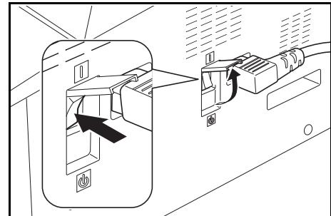
**Caution** ALWAYS turn the main switch to the scanner OFF BEFORE connecting the network cable.
